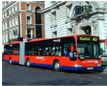
In 2003, London began introducing bendy buses. At 18 metres long, these vehicles can carry 140 people, at least 60 more than a double deck.
